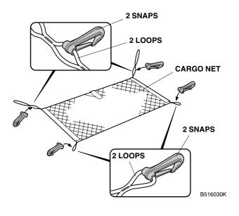
2. Install the cargo net to the tie-down hooks in the trunk as shown.
