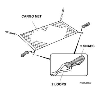
2. Install the cargo net to the anchors and tiedown hooks in the trunk as shown.
